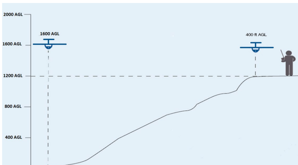
FIGURE 1 - SHOWING MODEL AIRCRAFT AT TAKE-OFF LOCATION OPERATING UP TO 400FT AGL, AT A SLOPE OF 1200FT ELEVATION
