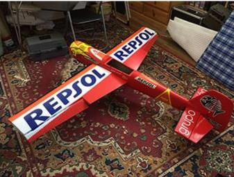
Running my hand over the paintwork, I could feel the ridges between the colours produced by the masking. Lightly rubbing down the model with 1200 grade wet and dry, used wet, has removed all the ridges resulting in a nice smooth finish. Now I just need to add the top varnish coat and that will be it. Back to Eastern Auto Paint for their recommendations.
