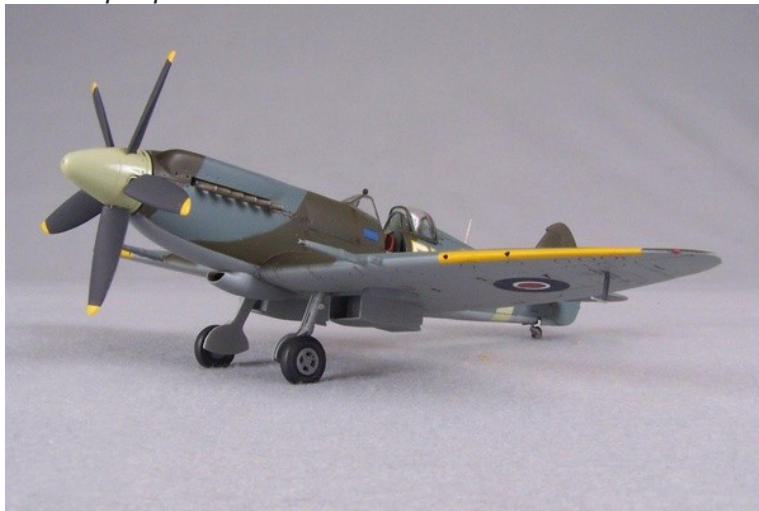
Spitfire Mk.XIX, with a 5-bladed propeller. The Mk.XIX had a Rolls-Royce Griffon engine which was a lot more powerful than the Merlin, hence the need for a bigger, more bladed propeller.
