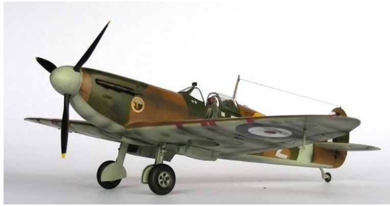
Spitfire Mk.II. Utilising a 3-bladed constant speed propeller.
