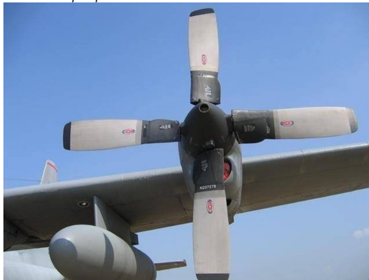
Later models of the C-130 used a 4-bladed Sabre design (if it can be called that).
