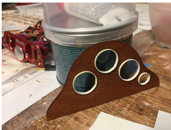
Left, the Avro Avian's instrument panel with the bezels from plasticard cut to length and superglued in place. If any of you have alternative methods for producing Instrument panels and would like to share your methods, please feel free to email me and I will include it in the newsletter.
