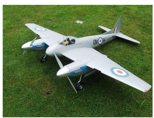
contra rotating props. All up weight is approx 10.5Kg. Maiden flight by Damien Mould showed it was somewhat underpowered. Recalibration of the ESCs solved that issue. Combined power from the two motors is now approx 2700 Watts so in excess of 115 Watts per pound. The next test should see significant improvement.
