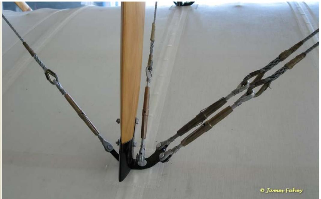
The Ultimate in Scale Modelling. The Vintage Aviator's replica BE2c (Early) - Specifically the base of the Starboard Inner Rear Interplane Strut. Here you can see the ouboard flying wires, the Inboard Land wire and the base of the interstrut bracing wire.
