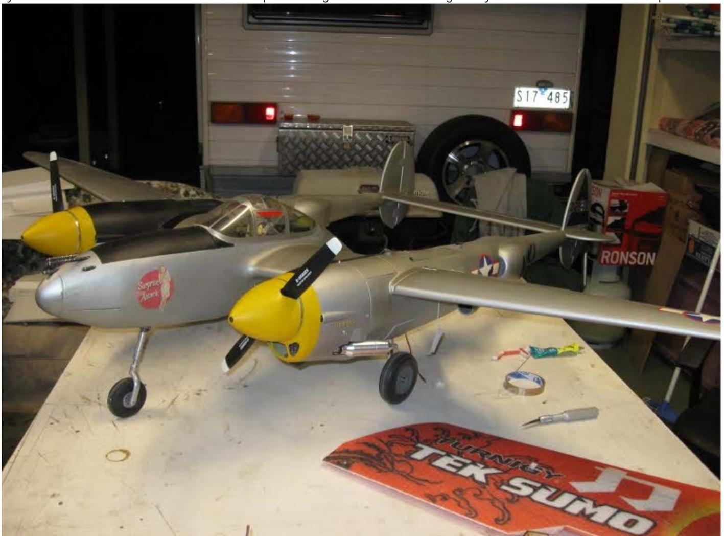
I hope to enter it on the next Haydn Hampson day. Details are 79 inch w/span, 2 FS 70 OS Engines, Robart retracts, Flaps, numerous servos and the most important part a naked lady on the nose!
