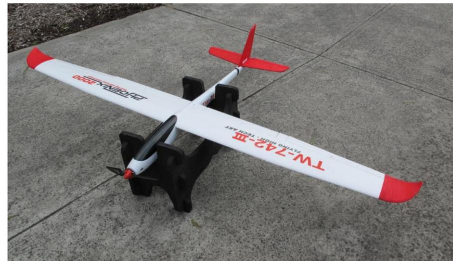
All of the foam components were well moulded and nicely finished but like too many Asian design products just a little clumsy. As an example, one can dismantle the wing into two pieces for store or transport but doing so involves small screws which would undoubtedly go missing at some point.
