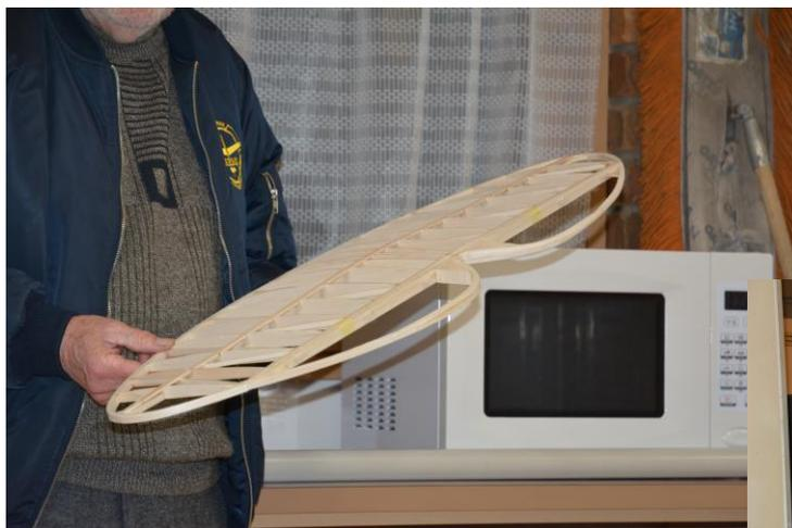
David Hipperson brought along his latest update to his “Mercury”. Converting a free flight model to an RC model requires David to ass things like Elevators, so he also strays from the kit structure somewhat in order to cut down weight. The structure in this case is a laminated outline supported by a braced framework.
