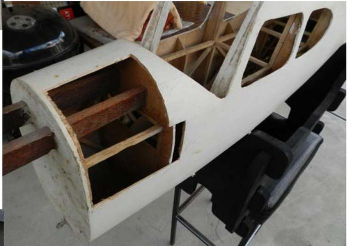
The balsa appears to be in reasonable condition and luckily the structure although light is very robust but that does not mean I'd take it at face value. Both the fuselage and wings are planked or sheeted as appropriate and then covered with some sort of lightweight filler. It was obvious that the model had been finished at some point but then stripped back prior to this filling which was all very odd. The fuselage
