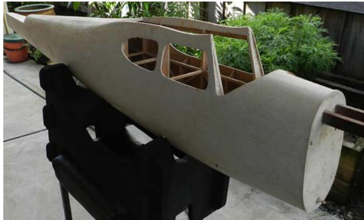
had some hole and cracks showed through the filler where I suspect it had simply just dried right out.
